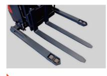
Straddle leg Adjustable straddle leg design, suitable for diverse pallet sizes and more stablity.
