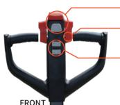
Emergency-reverse &Horn Buttons Dual butterfly-style thumb driving controls
