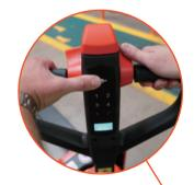
The function of driving with tiller in the **vertical position** helps with work in confined area without sacrificing of safety.
