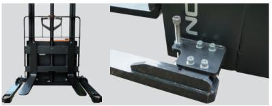
The support legs are fixed with screws located outside of the truck's body (4 screws for each side). The position can be easily adjusted according to the customer's needs to achieve the overall width of the truck: 46.5"/50.5"/54.5" 58.3".
