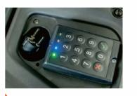
The option of PIN-code panel access, which works not only with PIN-code but also with access cards (RFID), can significantly simplify the procedure of access limitation for the fleet which may be used by more than one operator.
